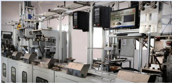
*The End of Line Test station ensures correct performance of every caliper we produce.*
