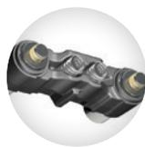
Twin return springs with a unique actuation block helps eliminate caliper or lever binding.
